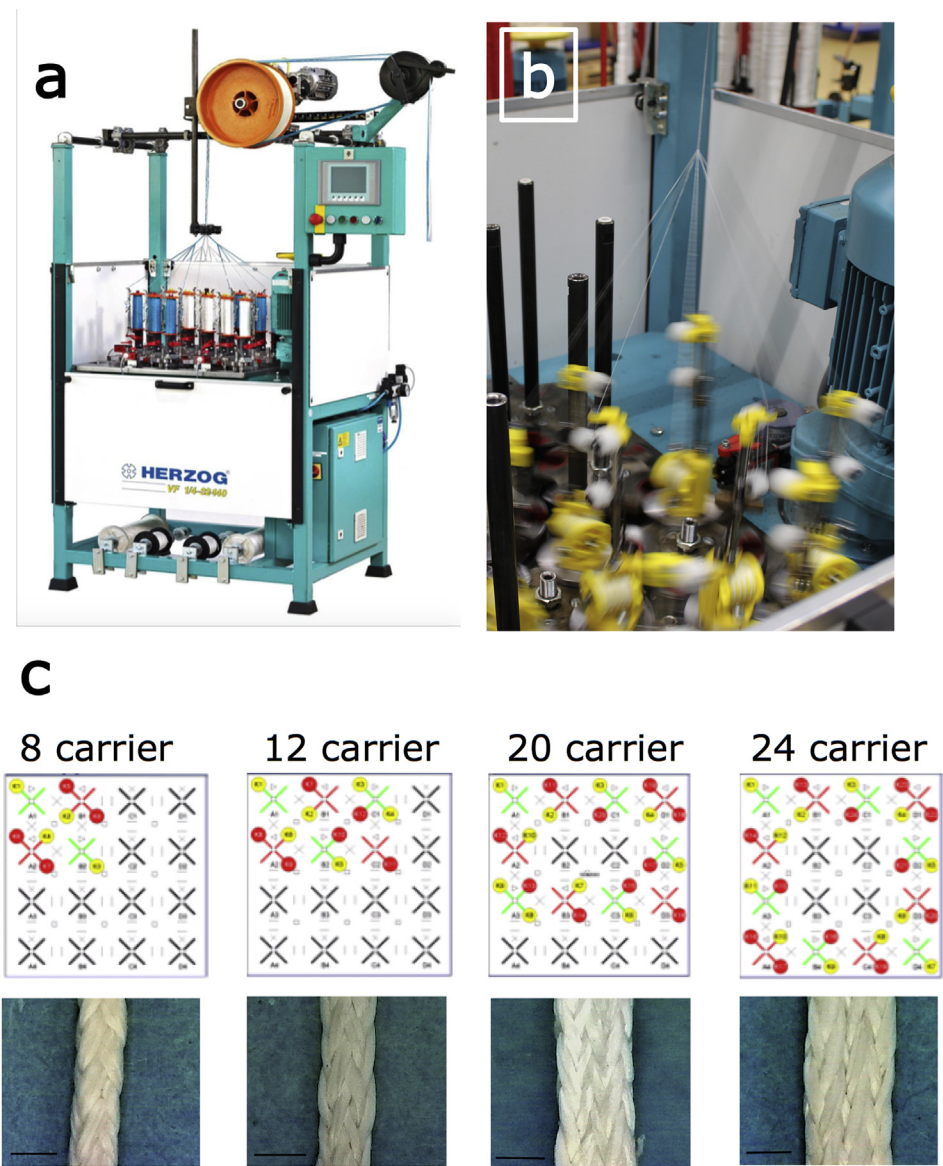
Fig. 1. Assembling multifilament electrospun yarns with an industrial braiding machine. (A) Variation Braiding Machine used to fabricate braided yarns. (B) Electrospun filaments being braided into a continuous yarn. (C) The various carrier arrangements used for manufacturing are shown above, and optical microscope pictures of the final yarns are shown below. Scale bars are 500 \mu m. It can be noted that the 8 and 12 carrier arrangement form a closed structure, whereas the 20 and 24 carrier arrangement form an open structure with a hollow centre.
